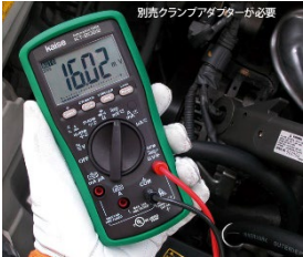
Alternator charging current
